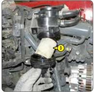
In case of use in a heavily dust laden atmosphere, there are pre-filtration cartridges, (< FILTER ELEMENTS AND BELTS). Also, the checking and cleaning periodicity of the cartridge must be reduced (up to 250 hours in a very dusty atmosphere and with pre-filtration).
