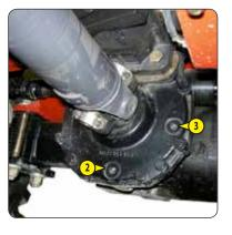
Place the lift truck on level ground with the engine stopped and the still warm differential oil.
